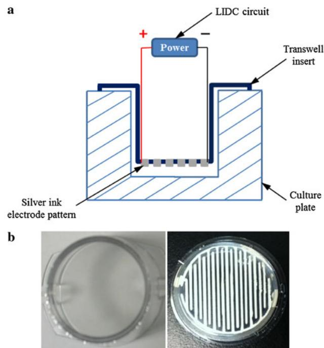
**Fig. 1** **a** Schematic of electrode testing configuration in a cell culture plate. **b** Blank Transwell insert (left) and silver ink printed onto the bottom of Transwell insert (right)
