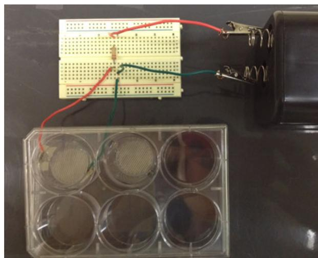
**Fig. 2** Overview of apparatus, showing six-well plate, battery and waffle board, all mounted on an acrylic plate. Silver electrodes printed onto the bottom of Transwells in *upper left* well (with 28  $\mu\text{A}$  current applied) and in *upper middle* well (no current applied), with an open well control in *upper right*
